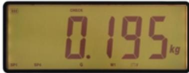
The color of the backlight, in the tolerance control function, automatically changes depending on the weight.
